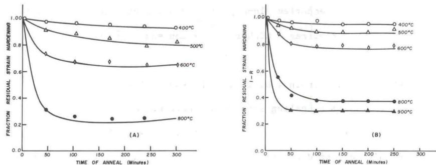
Figure 1 Isothermal recovery curves for shock deformed Fe-Mn, (a) 90 kb (b) 300 kb,
